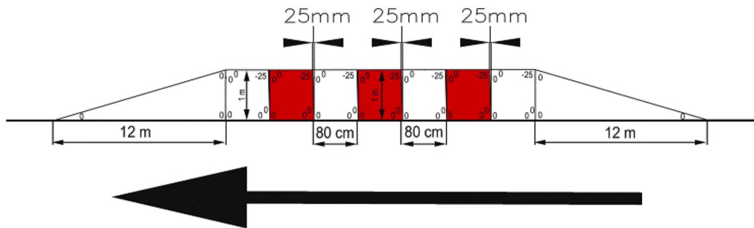
The 12 m triangle kerb at the beginning and the end of the kerb must be painted in white colour.
