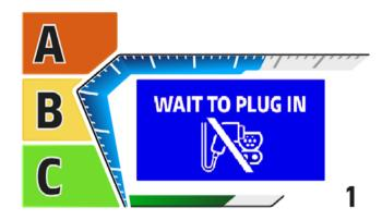
Wait until the message "Wait to plug in" disappears from the dashboard. Then to start DC charging connect the motorcycle to the external coumn fitted with a Fast Charge plug.
