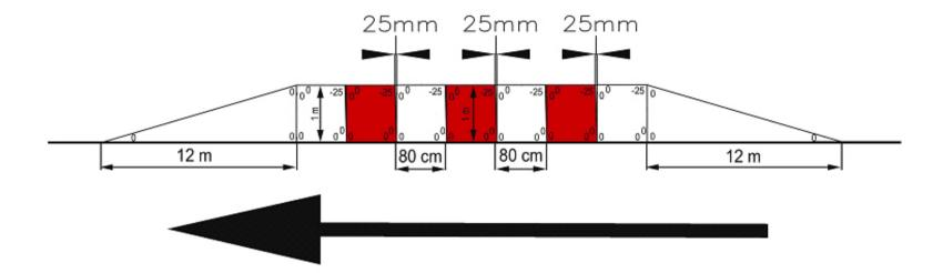
The 12 m triangle kerb at the beginning and the end of **the kerb** must **be** painted in white colour.
