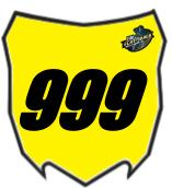
One plate must be fixed to the front inclined not more than 30° towards the rear from the vertical plane. Holes can be perforated between the numbers on the numberplate. However, under no circumstances must the actual numbers be perforated. The following minimum dimensions must be respected on the front number plate:
