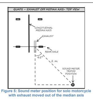
The sound level for engines with more than one silencer will be measured on each exhaust end.
