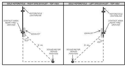
Figure 1 : Sound meter position for solo motorcycle
