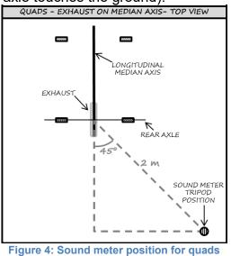
**for Quads with the exhaust moved out of the median axis**: at an angle of 45° from the exhaust axis, on the offset side, at a distance of 2 m behind the vehicle (measured from the point where the line drawn perpendicular to the rear axle touches the ground).
