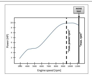
**For Trial**, the "max rpm" is established at 10000 ( $\pm$ 200) rpm and obtained thanks to a dedicated "sound test" mapping of the internal ECU or an external one, purpose-made and connected in occasion of the test.
