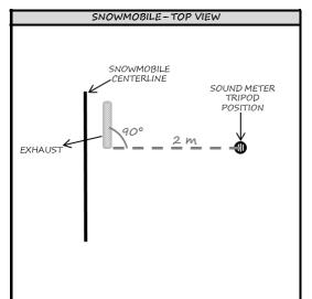
Figure 2: Sound meter position for solo snowmobile
