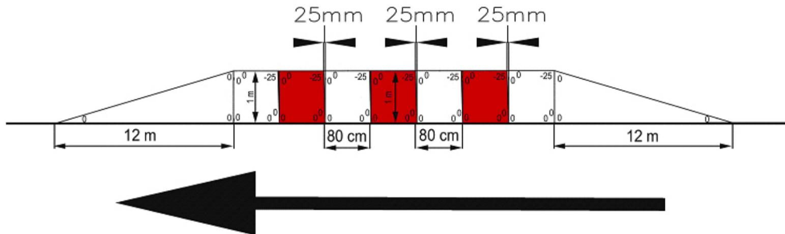
The 12 m triangle kerb at the beginning of the kerb and at the end of it must be painted in white color.
