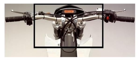
• TWO lights (like LED repeaters) must be visible from 10 meters away positioned on the both sides of the motorcycle (located in the identified area, please see the diagram hereunder). These two sides indicators must be protected from any possible contact (rider, environment, etc.).
