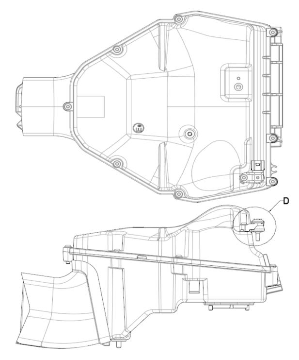
Moto2: Fig. 2: Ambient Air Pressure Sensor position
